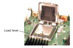
CPU installed in socket
